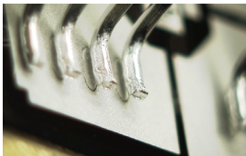
Degradations: detachment of connection wires
